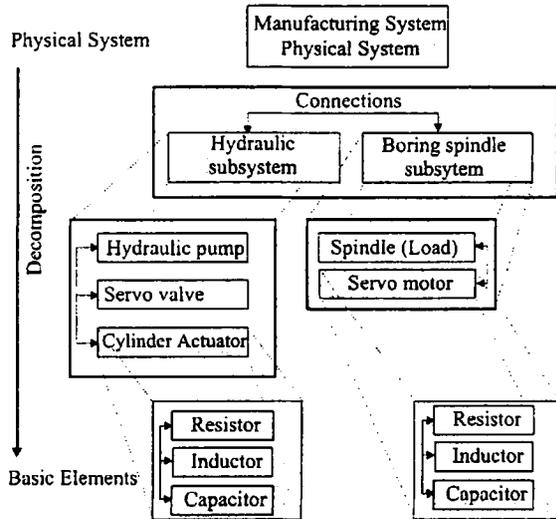
**Figure 3. Decomposition of the Physical System**
