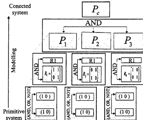
**Figure 6. Modelling of the Control System**
