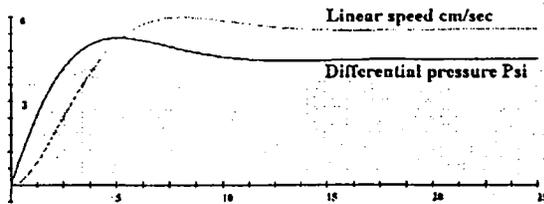
Figure 9. Linear Speed and Differential Pressure in the Actuator Cylinder
