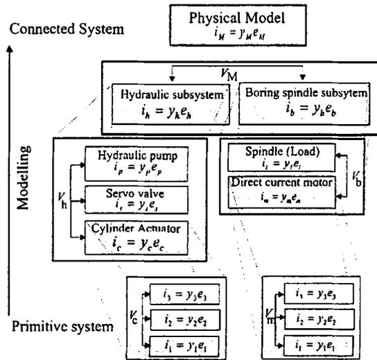
**Figure 4. Modelling of the Physical System**
