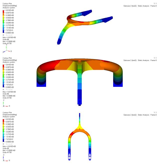
Subcase 2 (lateral impact simulation): the maximum displacement of the structure is equal to 6.8 mm, the maximum allowed value is equal to 17.5 mm.
